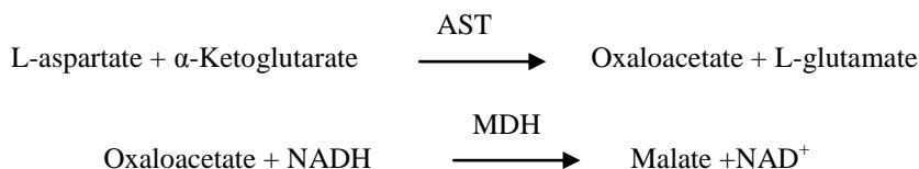
The rate of absorbance change caused by the conversion of NADH to NAD<sup>+</sup> is determined bichromatically at 340 nm and 405 nm. This rate is directly proportional to the amount of AST present in the sample.
